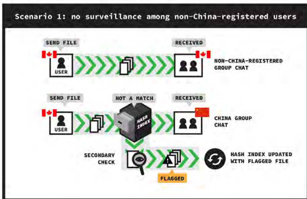
Figure 3: In the case of no content surveillance, the hash index is not updated when non-China-registered accounts send a novel, sensitive document to other non-China-registered accounts (top). Thus, when the same document is sent to China-registered accounts, the document is not censored (bottom).
