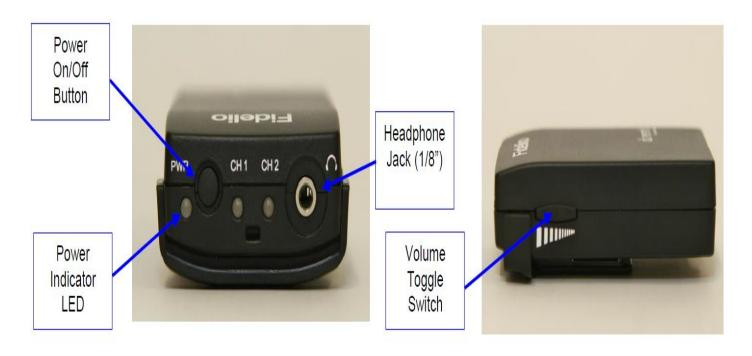
After the receiver is programmed, the employee will give you the receiver with headphones. Confirm that the VI LED light on the top of the receiver is on. It should be solid green or blinking slowly. You should also confirm that the power LED indicator is on and solid green, which means the battery is fully charged. You may either use the headphones supplied with the receiver or use your own headphones equipped with a standard headphone plug.
